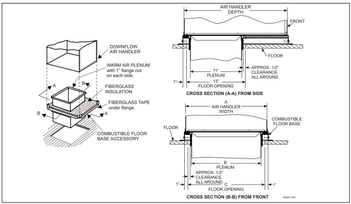
Figure 4: Combustible floor base accessory
